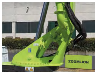
Turret with externally routed piping
