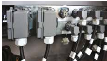
All aviation plugs are equipped with water and dust protection
